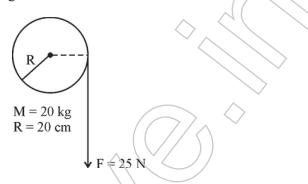
Calculate the angular acceleration of the wheel if steady pull of 25 N is applied on the cord. Moment of inertia of flywheel about its axis =  $\frac{MR^2}{2}$ .
